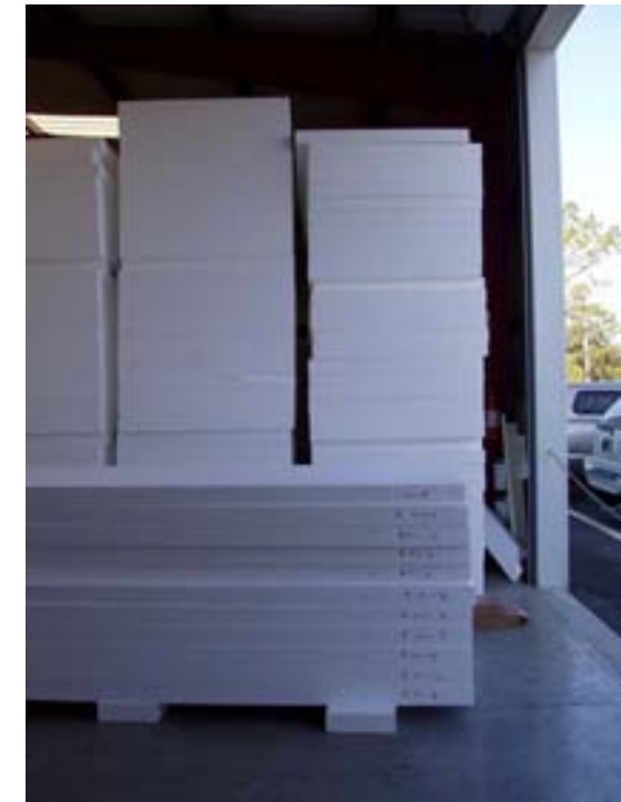
Foam cores drilled with utility chases for SIPs
