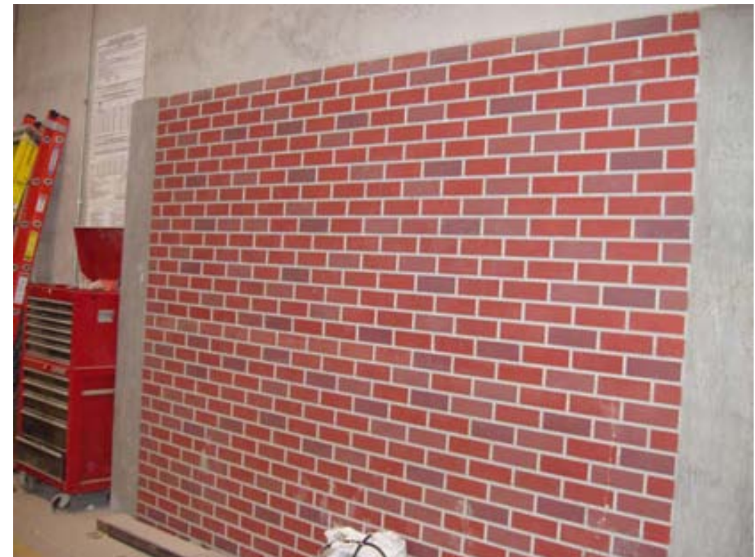
Insulated precast concrete panel is fabricated in Chicago with a brick exterior
