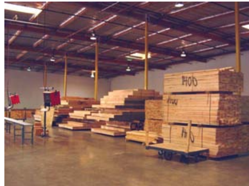
Raw materials ready for fabrication into wood-framed wall panels
