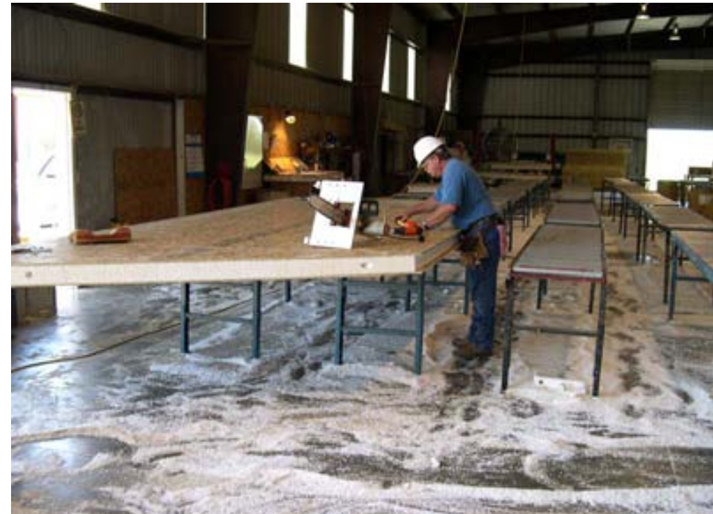
Window and door cutouts, along with angled profiles, can be made in the SIP plant
