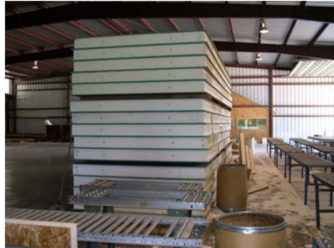
Structural insulated panels stacked prior to delivery; note pre-drilled chases for utilities
