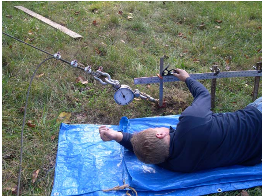
Figure 2.9. Deflection measurement technique for angle pull tests.
