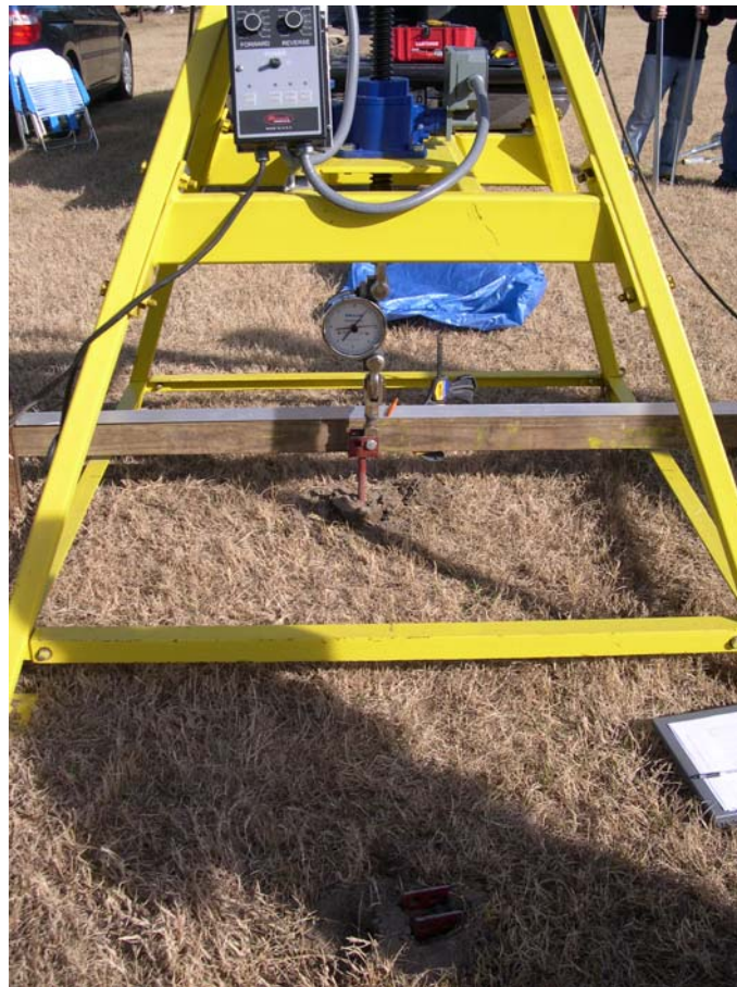
Figure 2.7. 90 degree in-line (axial) pull test set-up.
