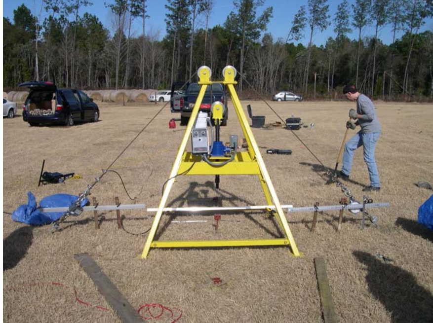
Figure 2.8. Angle pull test set-up
